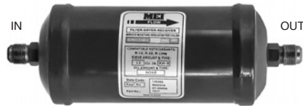
07-3055A Dia. - 3-3/4" Lgth. - 10-3/4" 41 cu.in. dessicant, 1/2" Male Flare TYPE AH414 In-Line Drier; TransAir A/C
