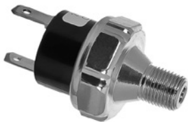
19-2605 Air Sensing Switch, N.C. Normally Closed, 1/8"-27 NPTF Open at 25 p.s.i.
