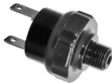
19-2608 Air Sensing Switch, N.O. Normally Open, 1/8"-27 NPTF Close between 20psi - 30psi
