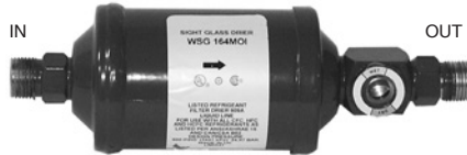
07-3063A Dia. - 2-3/4" Lgth. - 8-1/2" 16 cu.in. In-Line Filter Drier w/sight glass In - 1/2" Male Insert O'ring CARRIER # 14-00288-00; WSG164MIO
