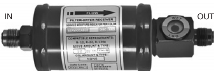
07-3064A Dia. - 2-3/4" Lgth. - 8-1/2" 16 cu.in. In-Line Drier w/sight glass In/Out - 1/2" Flare / O'ring; WSG164 FO
