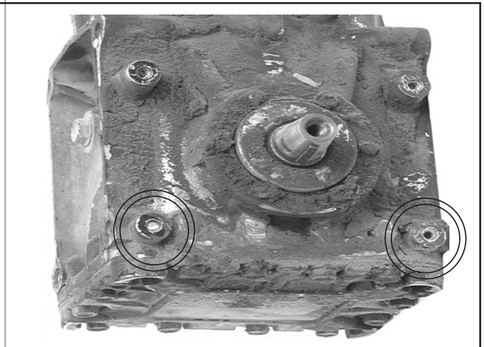
Stripped, broken or damaged clutch mounting threads.
