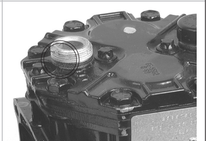
Dropped Compressor shown by the flat dent in threads.
